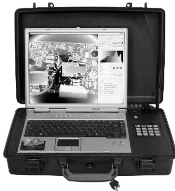
PC Based Control and Processing Unit
